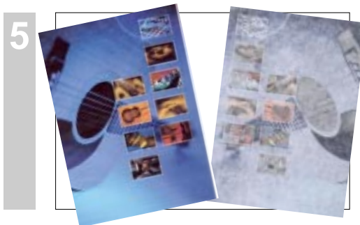
Printed side of Plain Paper Ink spreads, Sharpness lost
