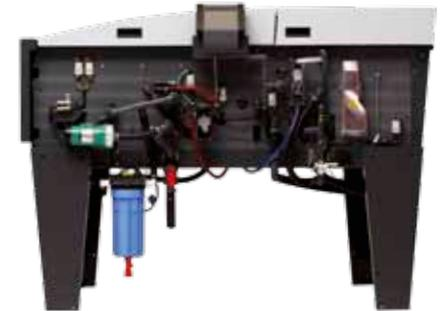
Keep your prepress room tidy by storing containers and auxiliary equipment under the processor. Can be easily covered with fitted side panels.
