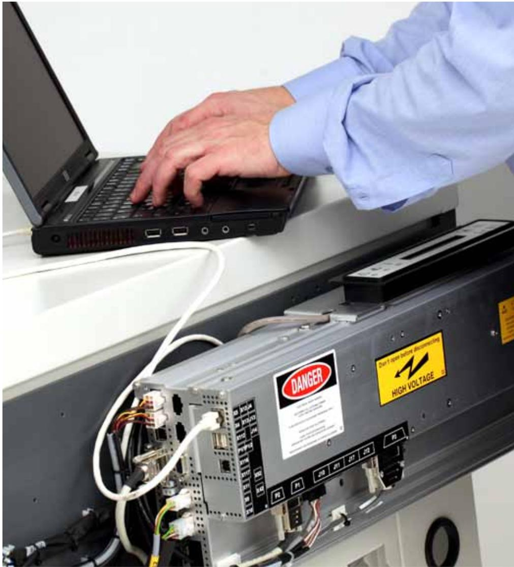
Glunz & Jensen's Remote Enabling System is included as standard and is used to configure the processor and allow for convenient remote service access via the internet.
