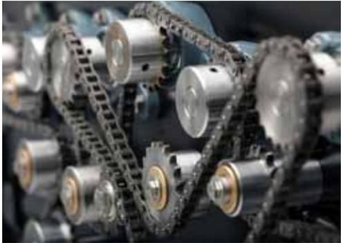
The Gecko+ 125 uses a traditional chain drive for rollers and brushes.
