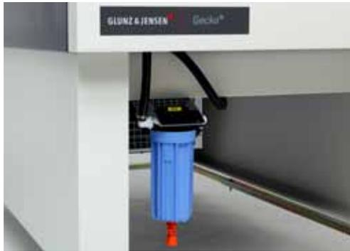
The filter house is conveniently mounted under the frame, giving easy access to the cooling unit and extra storage space for containers.
